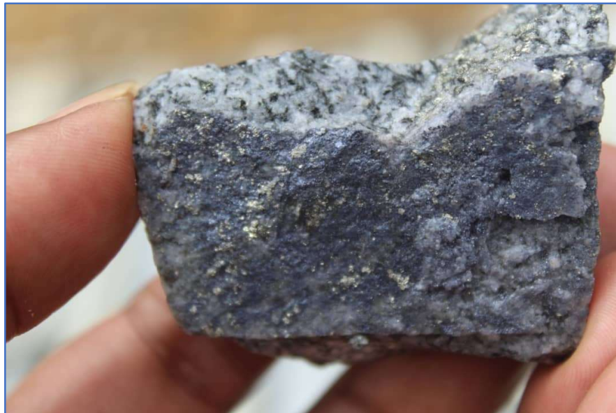
Figure 4. Rock Chip sample (MCRC_005) fracture surface almost entirely coated covered with 2mm layer of Molybdenite ( \text{MoS}_2 ) trace iron pyrite and bornite also observed
