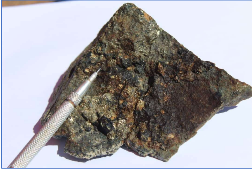
Figure 3. Rock sample (GGRC_004) from TRMC 13, Pyrite – chalcopyrite and bornite on a rock chip collected from a fracture surface, in this instance, a 3mm layer of sulphides covers 100% of the fracture surface, with the main sulphide minerals comprising ~95% iron pyrite, ~3% chalcopyrite and ~2% bornite.
