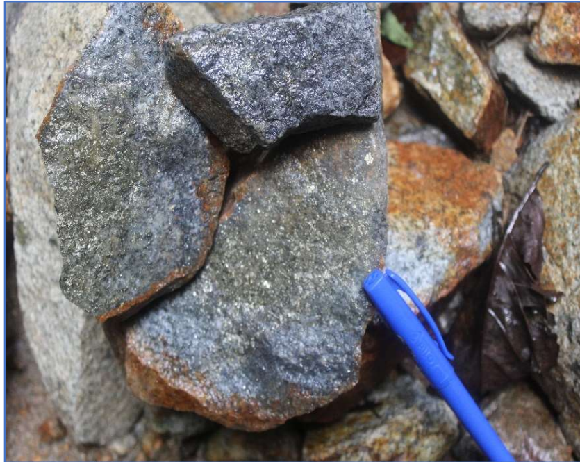
Figure 5. Rock chip sample (KBRC_003) from Kombanlam Creek, fracture surface coated with sulphide layer which is 2mm thick, sulphides are predominantly iron pyrite (~70%) and molybdenum (30%), with only minor dissemination of sulphides (1%) in the rock matrix.
