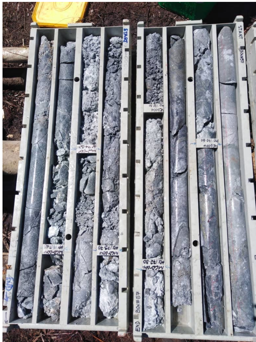
Figure 1. MCD004 – Core trays which contain part of the 8.4m zone @ 0.40 g/t Au, 0.22% Cu and 689ppm Mo
