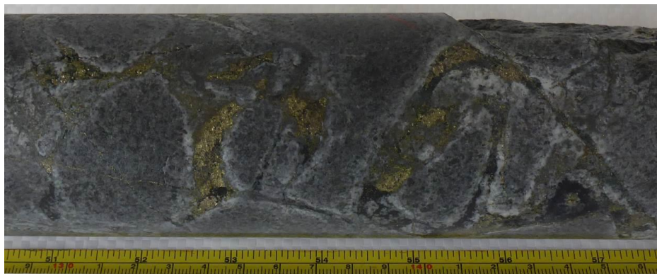
Figure 5 MCD002 189.80-189.98m: Brecciated tonalite with chalcopyrite ( \text{CuFeS}_2 ), pyrite, magnetite (black) and quartz cement (HQ Core 63mm diameter; scale: inches and centimetres)
