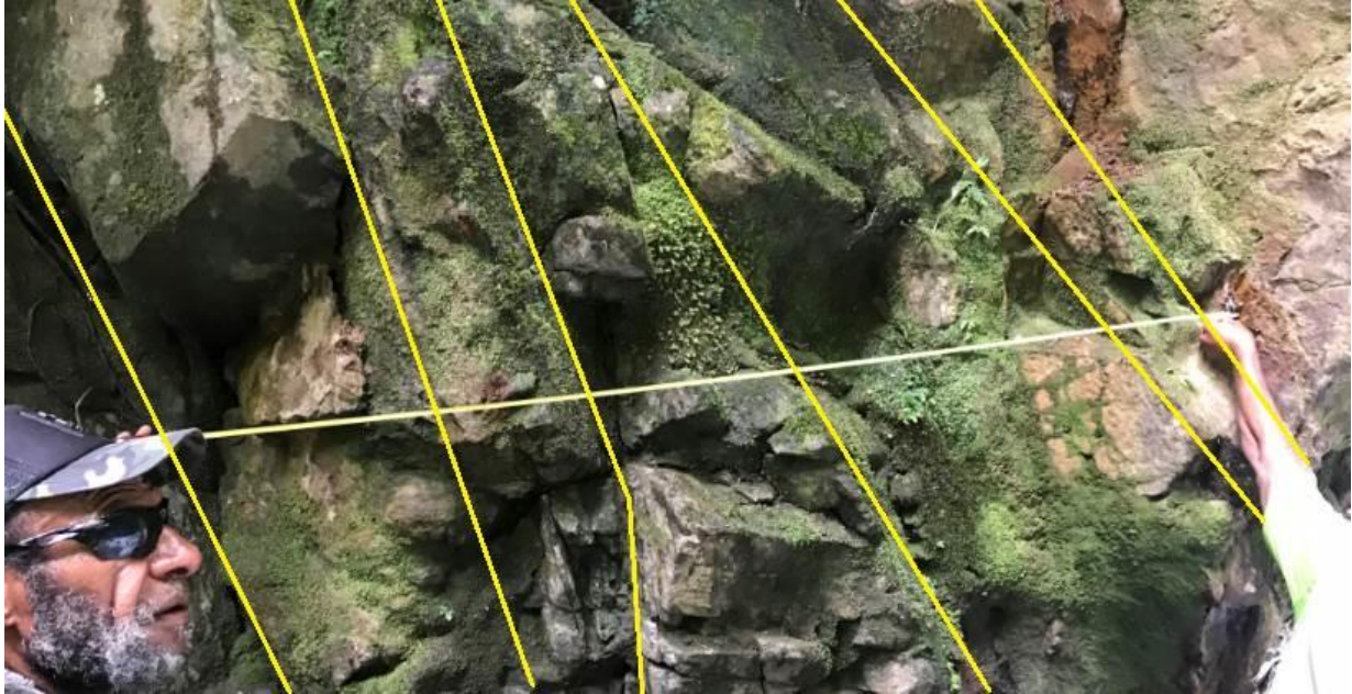
Figure 10: Yakari Creek -Kulinlam, location of vein which assayed 0.99% Cu and 0.1 1ppm Au. Photograph shows the 6 sub-parallel veins (yellow lines) which occur within a 2 m interval, (white tape measure).
