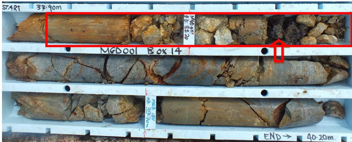
Figure 4 Photo of core box that includes the intercept at 38-39m, showing a ~10cm solid sulphide intercept running close to 10% Cu and 0.2% Ag.
