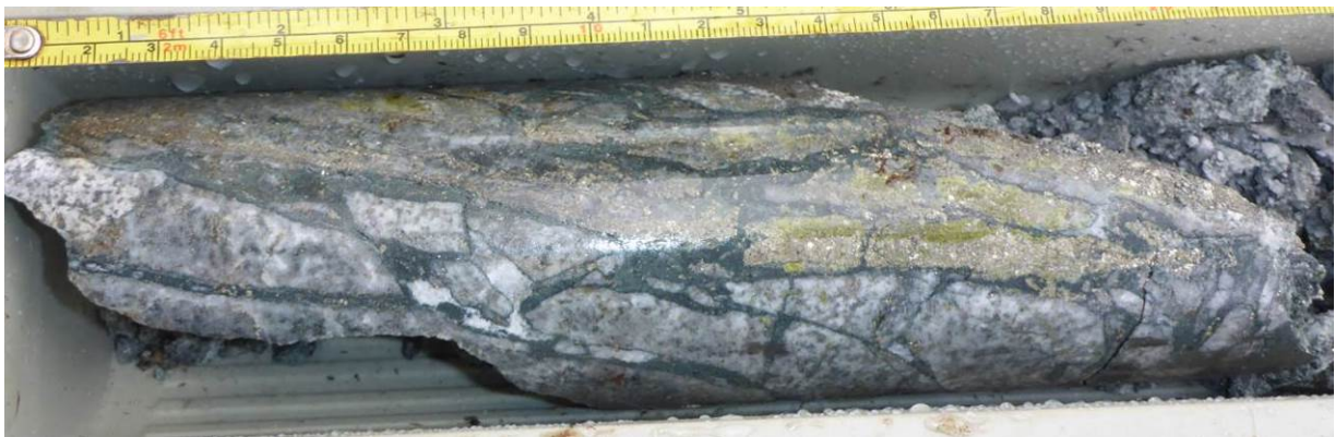
Figure 9. MCD001 - 317.6 metres downhole. Mosaic brecciated diorite with quartz-pyrite cement
