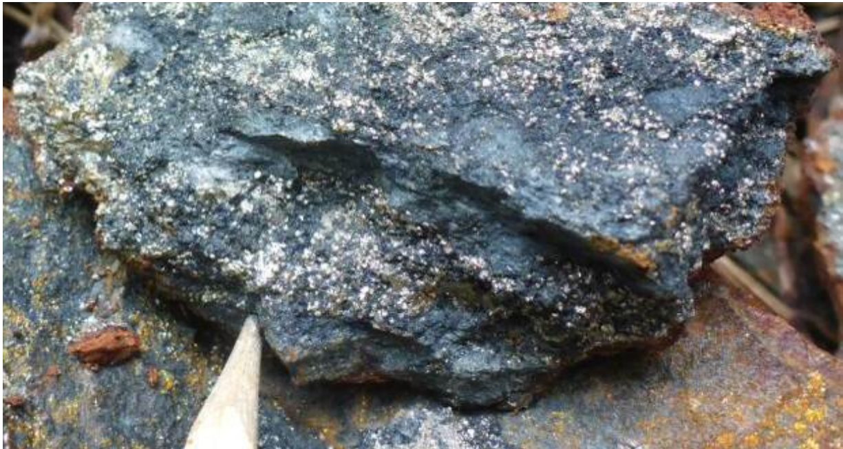
Figure 2. Porphyritic hornblende microdiorite float sample 41733: 0.59% Cu, 0.05 g/t Au. The rock has good preservation of primary porphyry texture and early, localised effects of potassic alteration are manifest in development of minor patchy biotite and actinolite, accompanied by minor magnetite, pyrite and trace chalcopyrite (pencil for scale).
