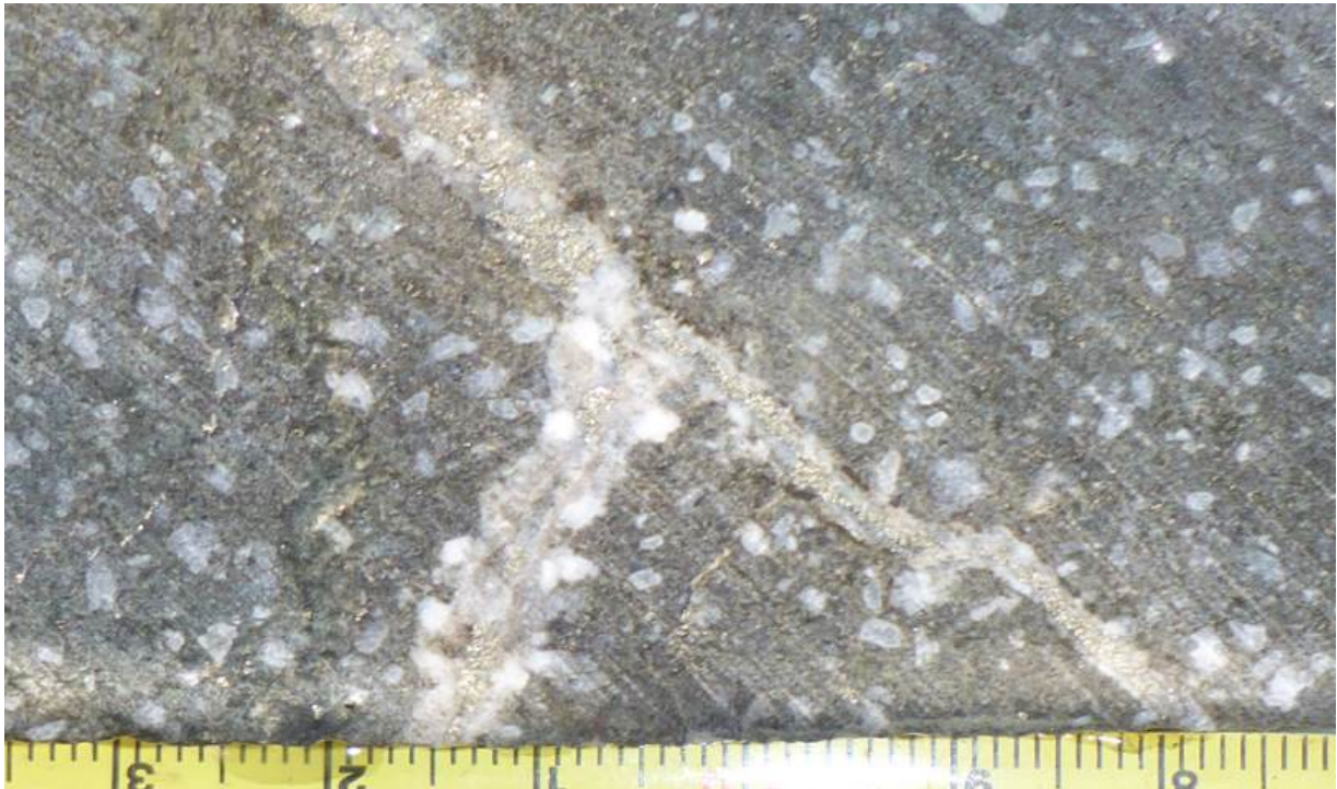
Figure 6. MCD001 - 124.7 metres down-hole. Quartz-sulphide veins in porphyritic diorite
