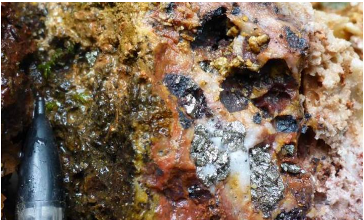
Figure 3 Silica flooded diorite float sample 41735: 0.44 g/t Au, 227 ppm Cu. Large (up to 10mm long) pyrite cubes. Note several partial dodecahedral and cubic vugs left after leaching has removed sulphides (pencil for scale).
