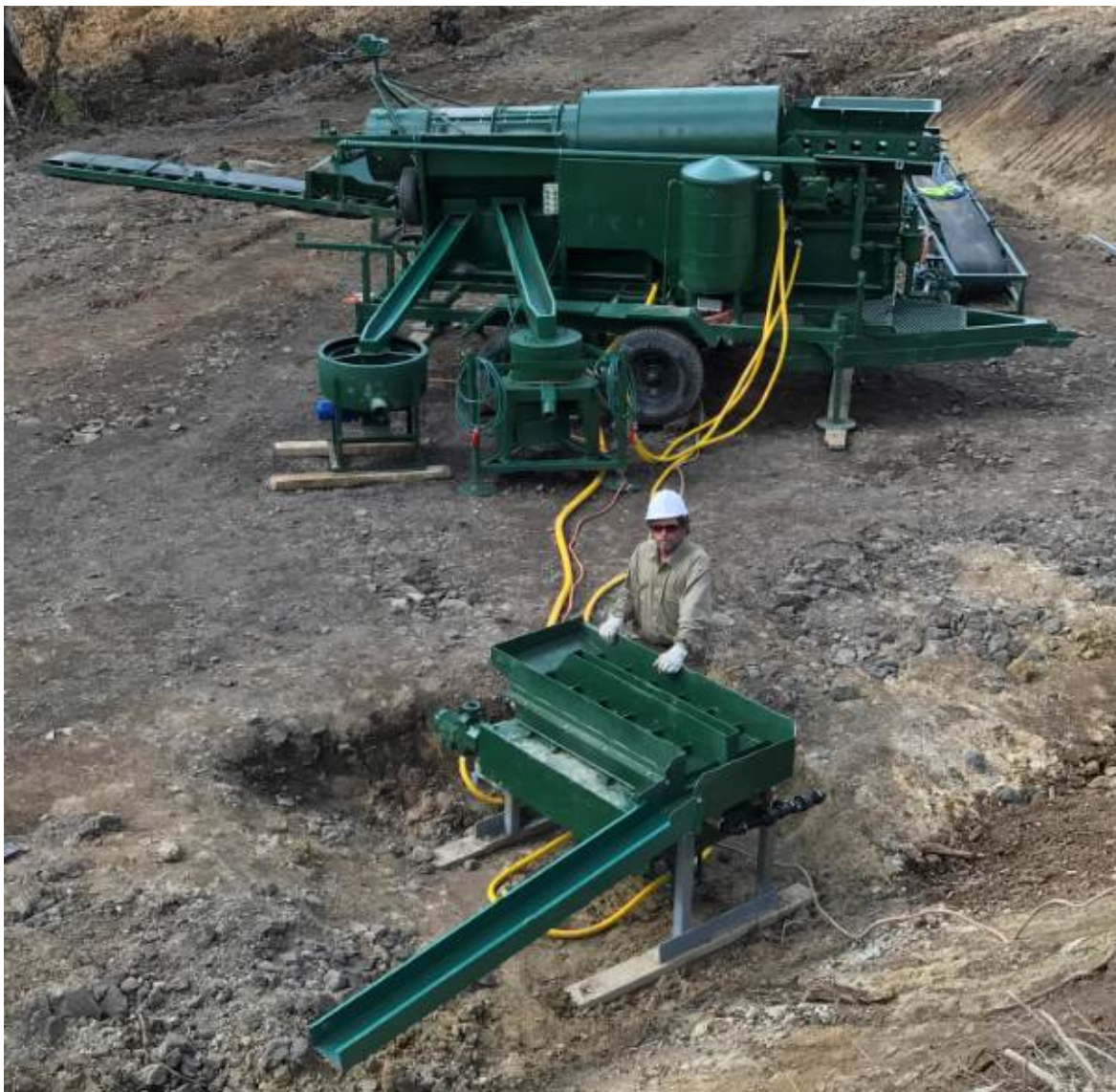
Figure 1: Gravity-gold-recovery consultant Ken Wilson standing beside pulsating jig, with trommel, Knelson and Knudson bowl in background
