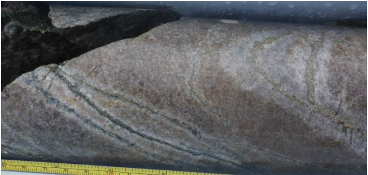
Figure 5: Detail of core in Figure 4 above showing earlier stage higher temperature reddy-brown potassic alteration overprinted by late stage pyrite-quartz veins (Diamond drill hole MCD001, refer to photo above for relative downhole depth. Scale: upper scale: inches; lower scale: centimetres).
