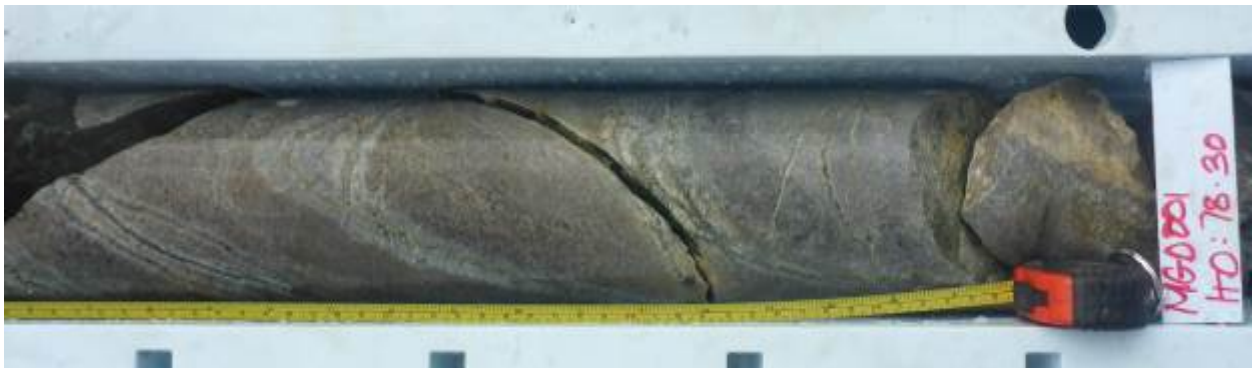
Figure 4: Potassic alteration (reddy-brown) overprinted by sheeted and stockworked pyrite-quartz veins with phyllic alteration selvages in microdiorite. Potassic alteration is a significant diagnostic characteristic of porphyry copper-gold systems (Diamond drill hole MCD001, RHS of core 78.30 metres downhole. Scale: upper scale: inches; lower scale: centimetres).
