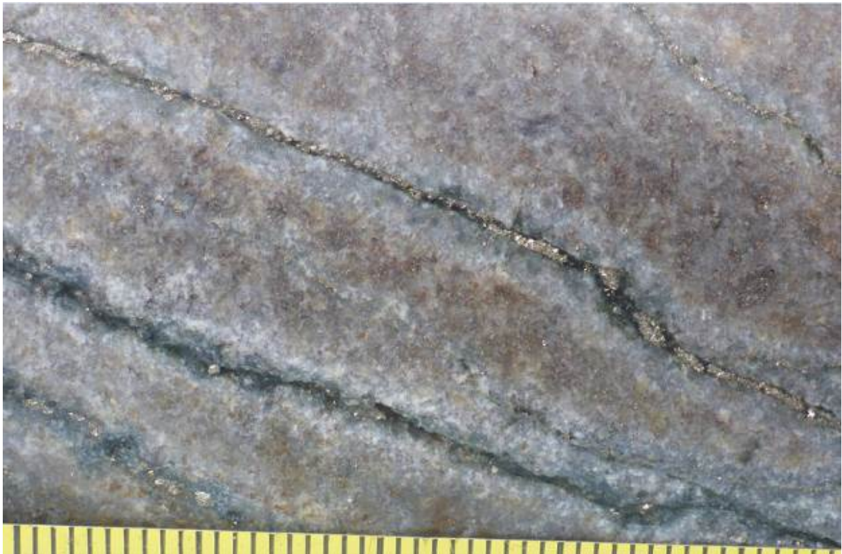
Figure 7: Detail of core in Figure 4 above showing earlier stage higher temperature reddy-brown potassic alteration overprinted by late stage pyrite-quartz veins (Diamond drill hole MCD001, refer to photo above for relative downhole depth. Scale: centimetres, millimetres).
