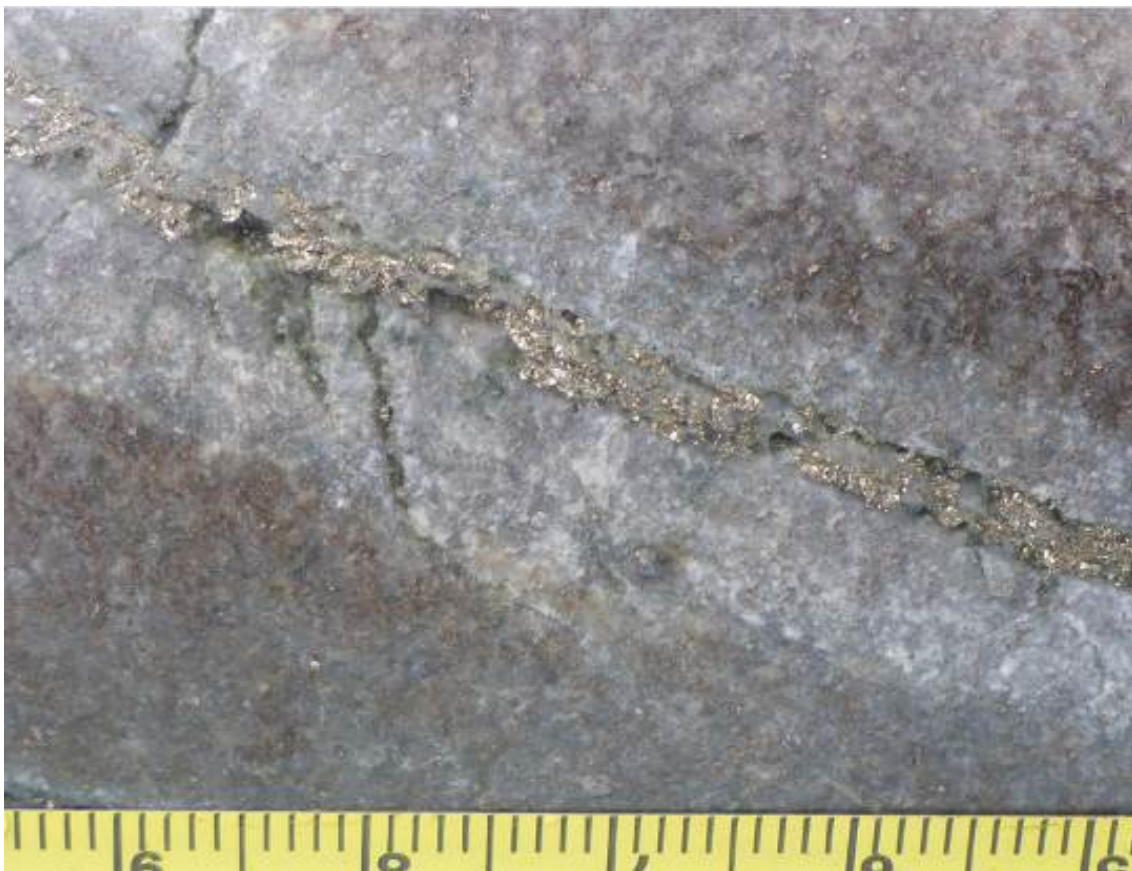
Figure 6: Detail of core in Figure 4 above showing earlier stage higher temperature reddy-brown potassic alteration overprinted by late stage pyrite-quartz veins (Diamond drill hole MCD001, refer to photo above for relative downhole depth. Scale: centimetres, millimetres)
