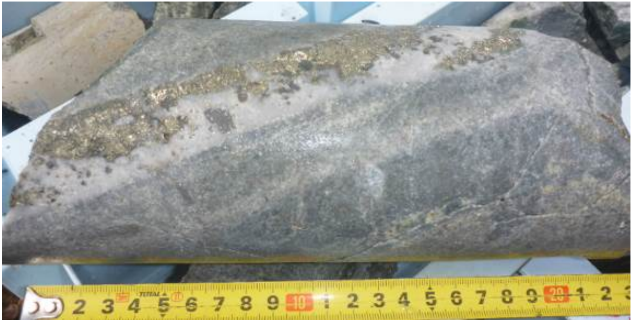
Figure 3: 4cm wide quartz-pyrite vein in phyllic altered microdiorite (centre of vein 77.7 metres down hole in Mongai Creek Porphyry Copper-Gold System (Diamond drill hole MCD001. Scale: centimetres, millimetres)
