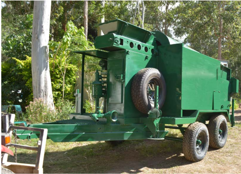
Figure 2: Mobile gravity gold bulk sampling plant engineered and constructed in Australia
