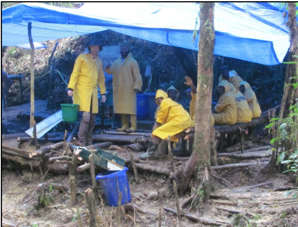
Figure 3: Processing of pit samples using a Knelson concentrator and sluice box to collect heavy mineral concentrates
