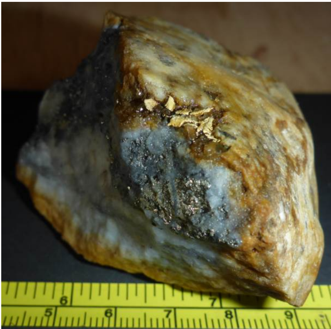
Portion of large quartz cobble containing crystalline dendritic and wire gold indicative of boiling zones of epithermal gold deposits. Scale in both inches and centimetres. Images following are enlargements of the bonanza-type crystalline gold, refer to scale in this photo for dimensions.
