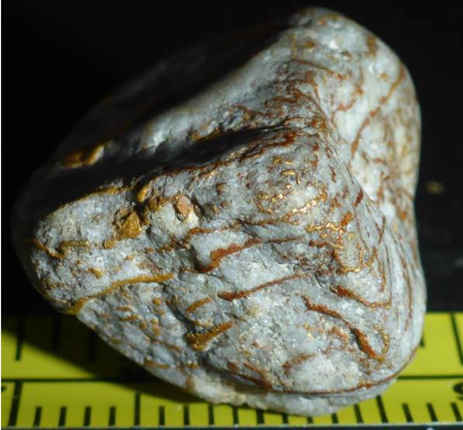
Wire gold clearly shed from a high grade gold source. Scale in both inches and centimetres.
