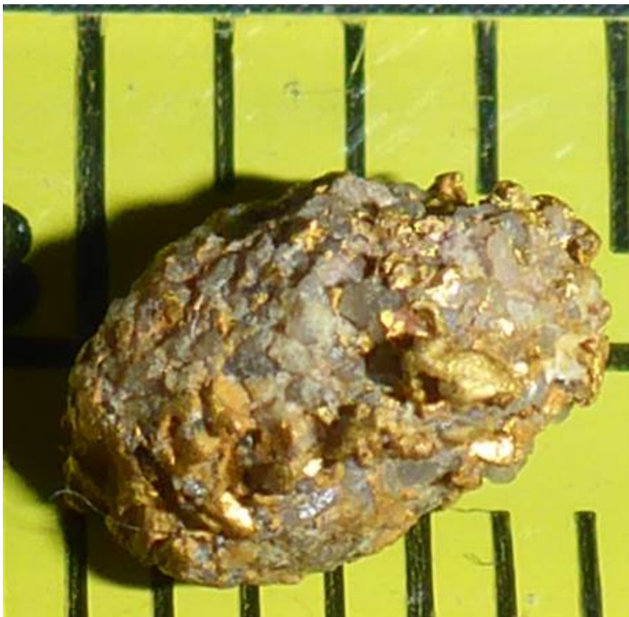
Crystalline gold and interlocking prismatic quartz. Scale in both inches and centimetres.
