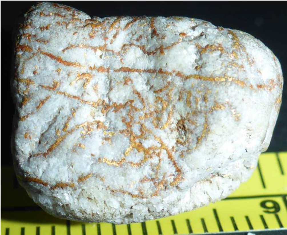
Wire gold clearly shed from a high grade gold source. Scale in both inches and centimetres.
