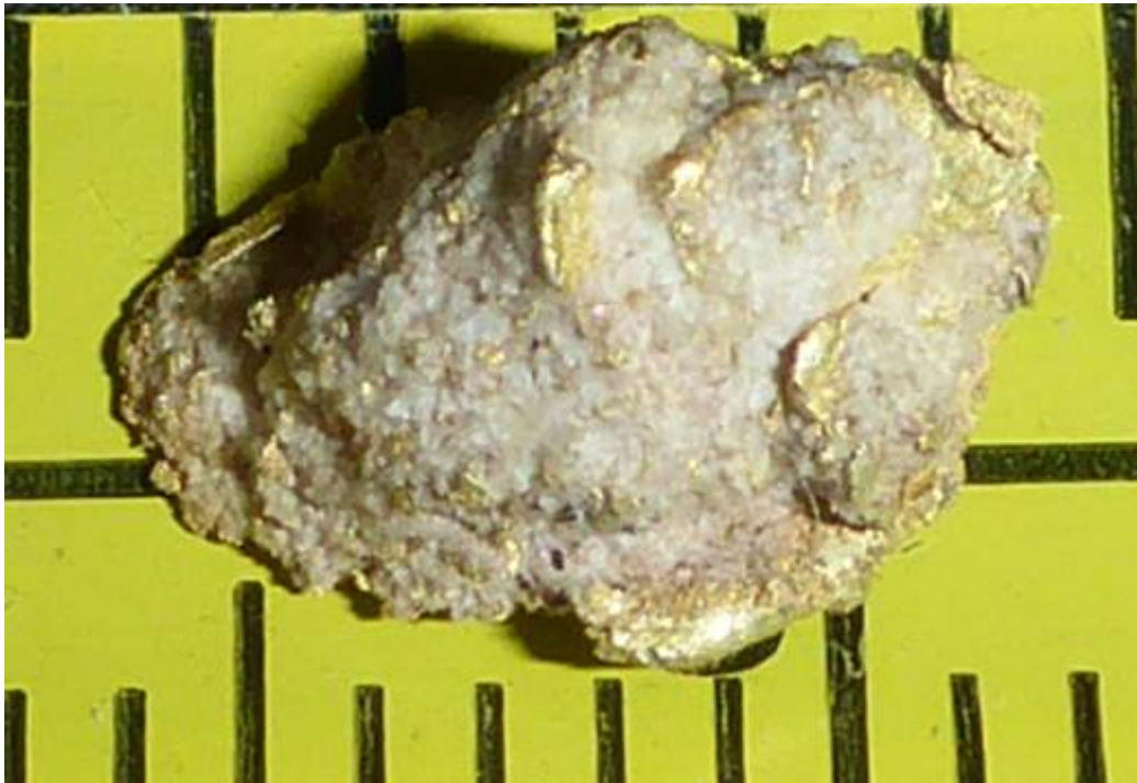
Crystalline gold and interlocking prismatic quartz. Note how the 'sugary' white quartz is friable and disaggregating to release the gold. Such a fragile specimen must be very close to its source. Scale in both inches and centimetres.
