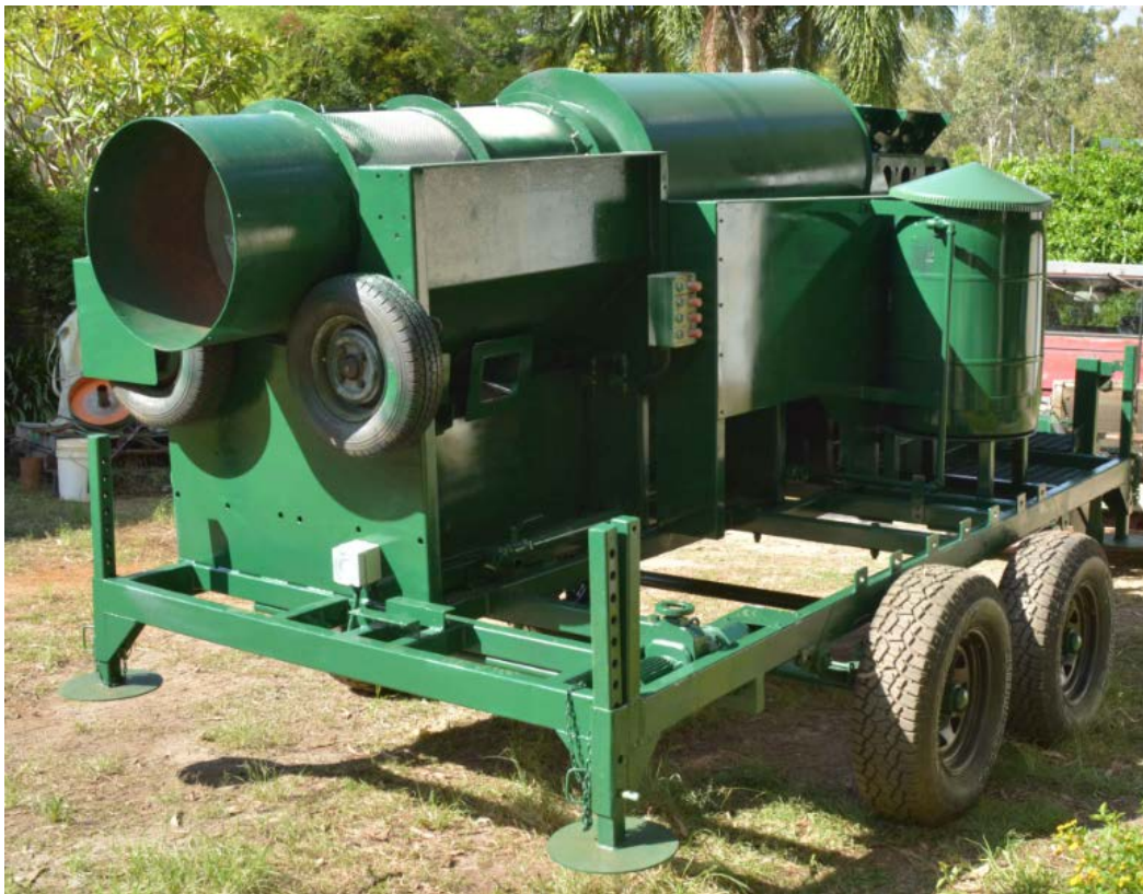
View of trommel and wet scrubber of mobile gravity gold bulk sampling plant
