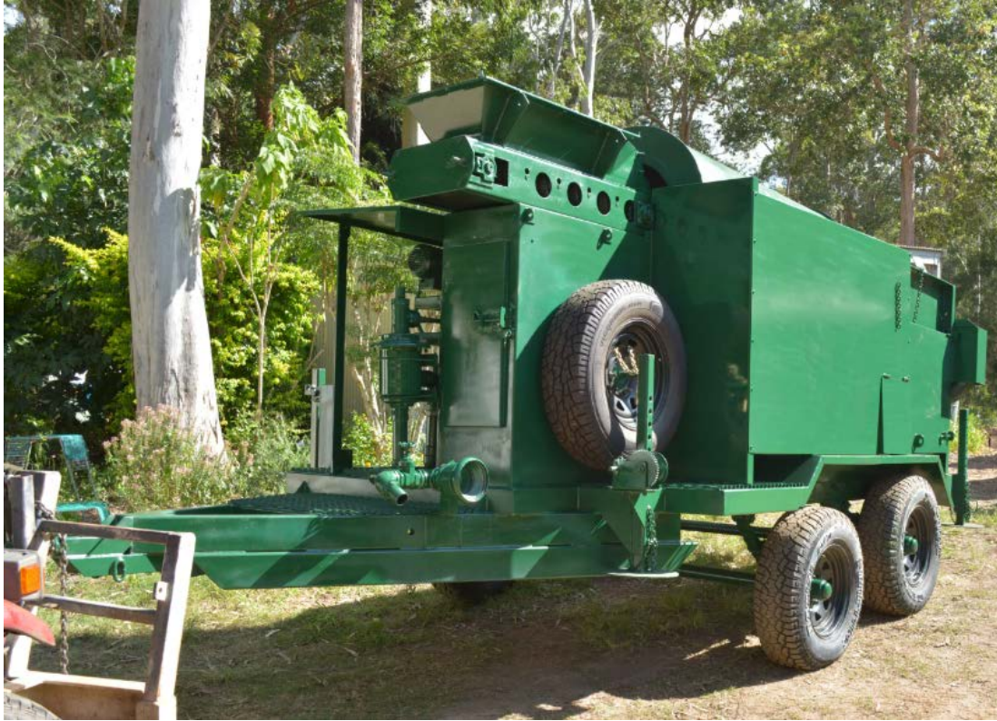
Mobile gravity gold bulk sampling plant was engineered and fabricated in Australia
