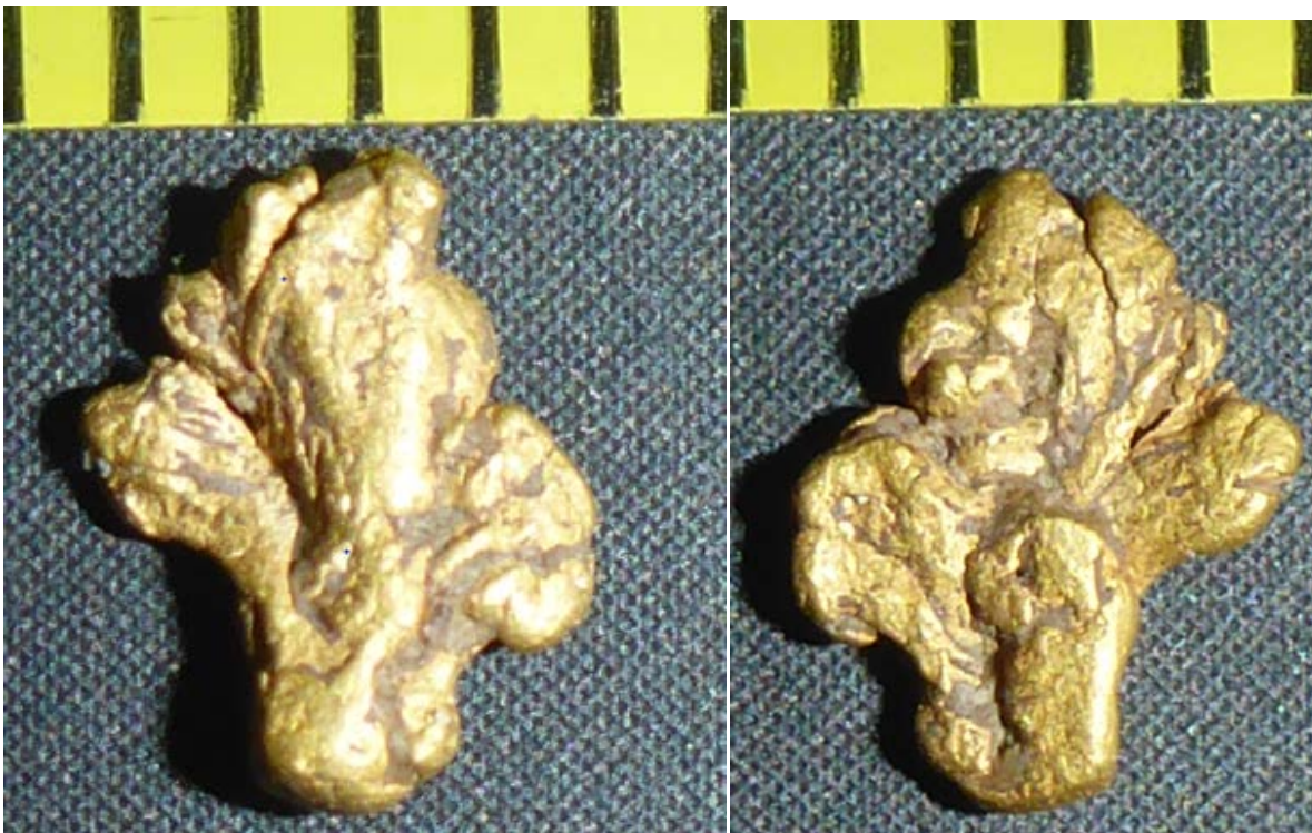
Photo 6: Dendritic Gold. Scale: Divisions in millimetres
