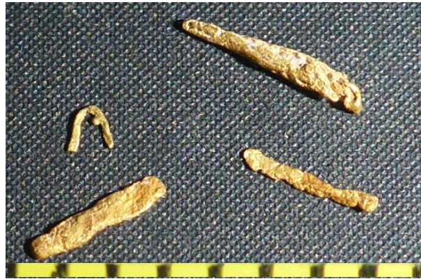
Photo 3: Dendritic gold (left), and Wire gold (right) – Crown Ridge 3 March 2018. Scale: Divisions in millimetres
