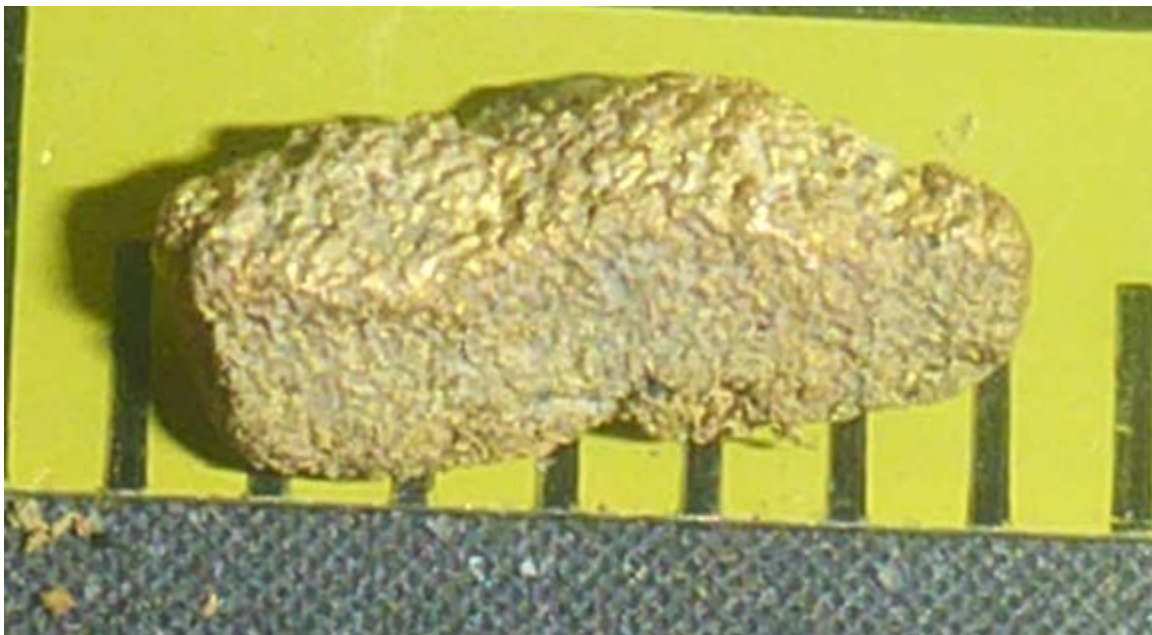
Photo 12: Gold exhibiting a mammillated surface and angular shape indicating it has undergone minimal transportation - Crown Ridge 3 March 2018. Scale: Divisions in millimetres
