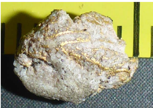
Photo 4: Dendritic gold (top), and wire gold in quartz (bottom) - Crown Ridge 3 March 2018. Scale: Divisions in millimetres
