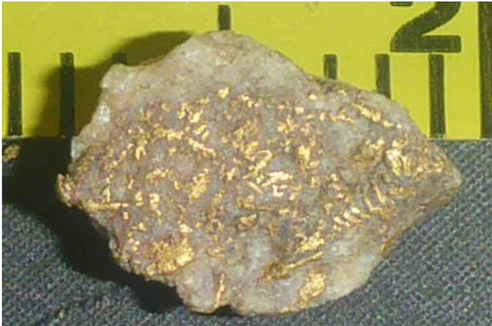
Photo 11: Dendritic and Wire Gold - Crown Ridge 3 March 2018. Scale: Divisions in millimetres
