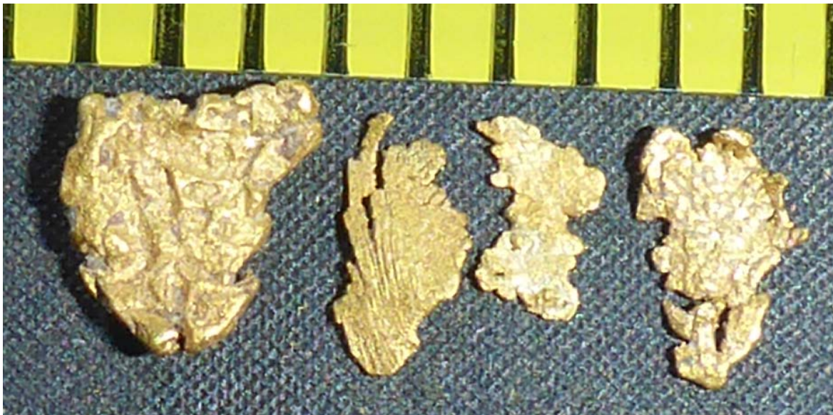
Photo 15. Two views of angular gold particles, some dendritic Gold. Different lighting intensities to highlight aspect of morphology - Crown Ridge 3 March 2018. Scale: Divisions in millimetres
