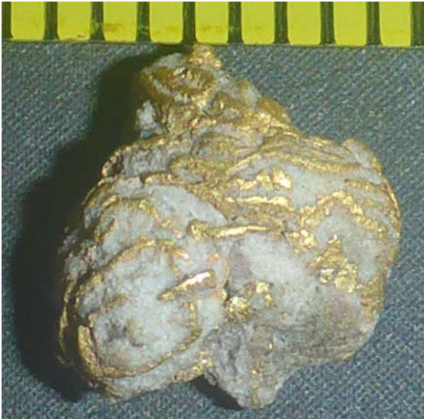
Photo 7: Wire Gold - Crown Ridge 3 March 2018. Scale: Divisions in millimetres
