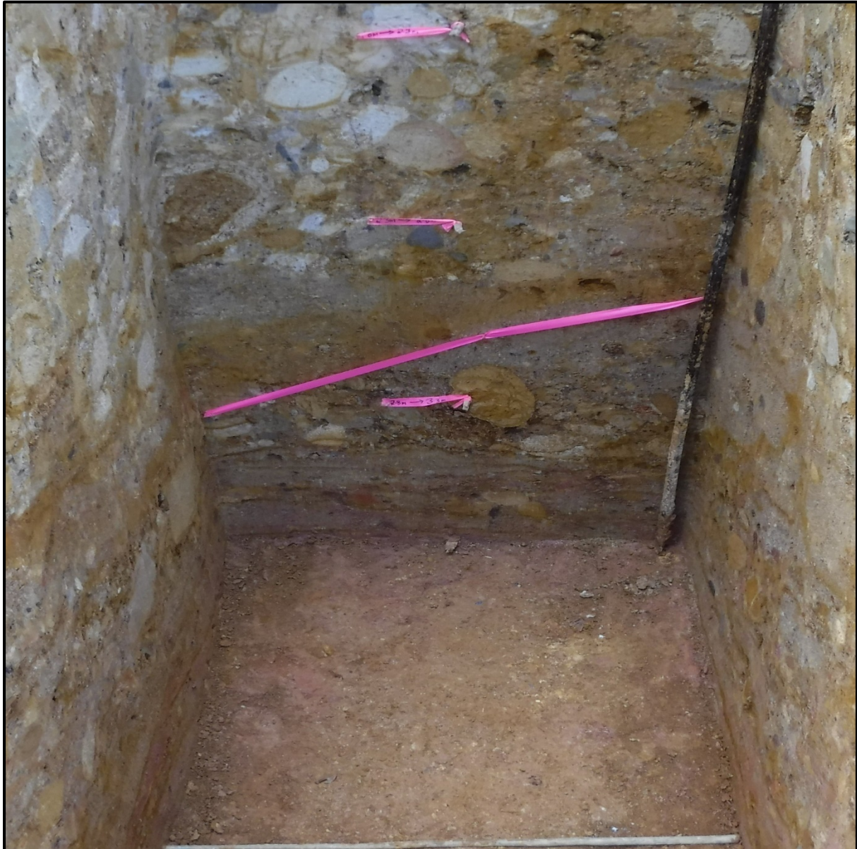
Figure 4: Photo of pit CRP001 showing altered and weathered conglomerate and interbedded sandstone units
