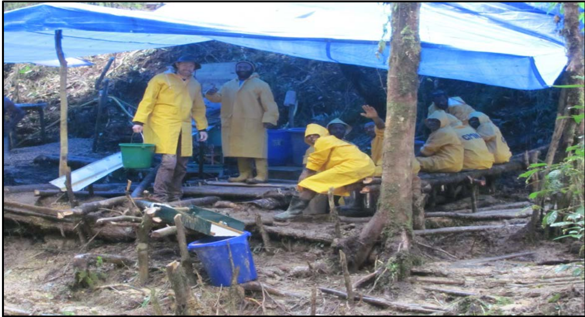
Figure 5: Processing of pit samples using a Knelson concentrator and sluice box to collect heavy mineral concentrates
