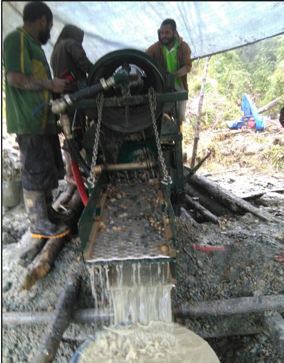
Photo 2: Portable heavy mineral test plant processing material to produce a concentrate
