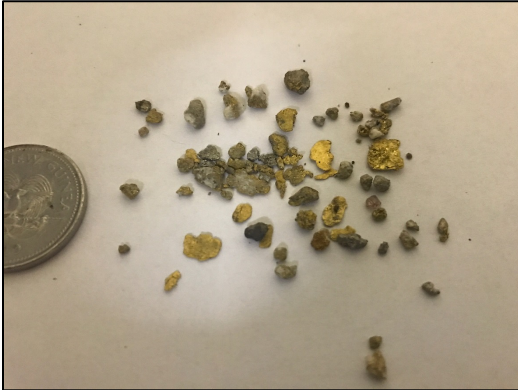
Photo 3: Coarse gold particles and gold-quartz vein material from the trommel oversize (diameter of coin approximately 28mm)
