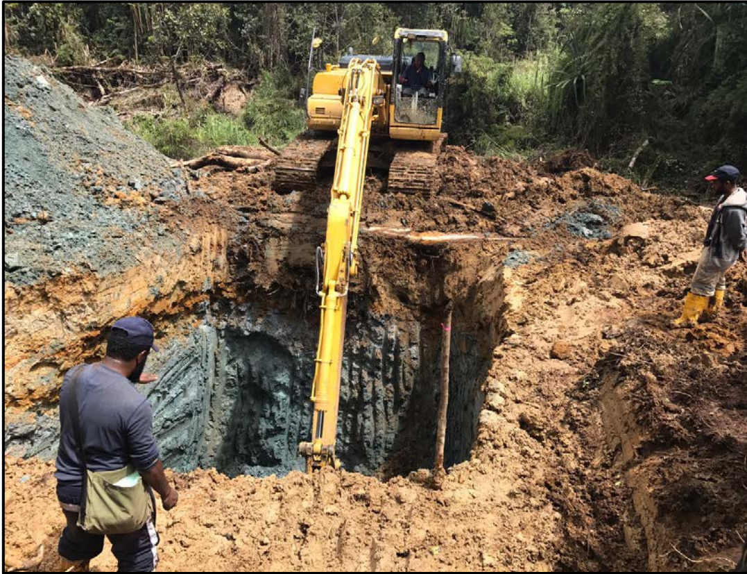
Photo 1: Excavator digging bulk sample pit at Crown Ridge
