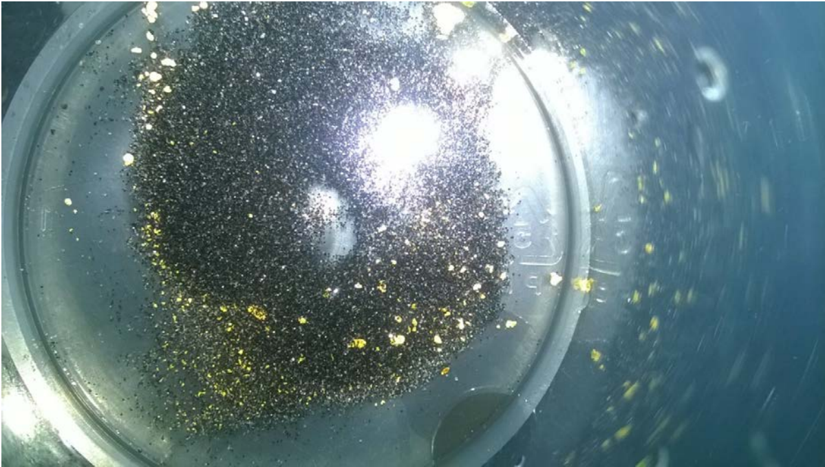
Figure 11. Pit 31 visual gold in panned concentrate (Photo from ALS Metallurgy Pty Ltd, Perth).
