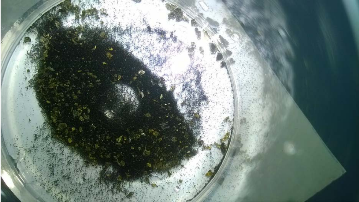
Figure 9. Pit 18 visual gold in panned concentrate (Photo from ALS Metallurgy Pty Ltd, Perth).
