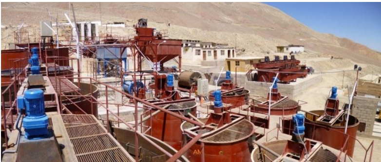
Photo of the Mollehuaca Gold Plant: leach tanks (left; taken on 3/9/2013) and tailings field (right; taken on 26/10/2013)
