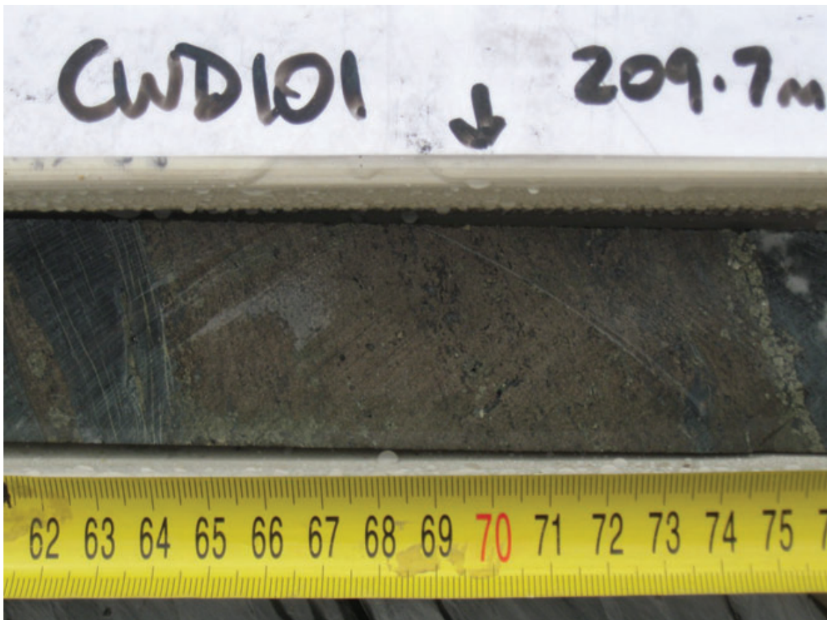
Photo 2: Massive pyrite-pyrrhotite vein, Independent Lode, CWD101: 209.7m
